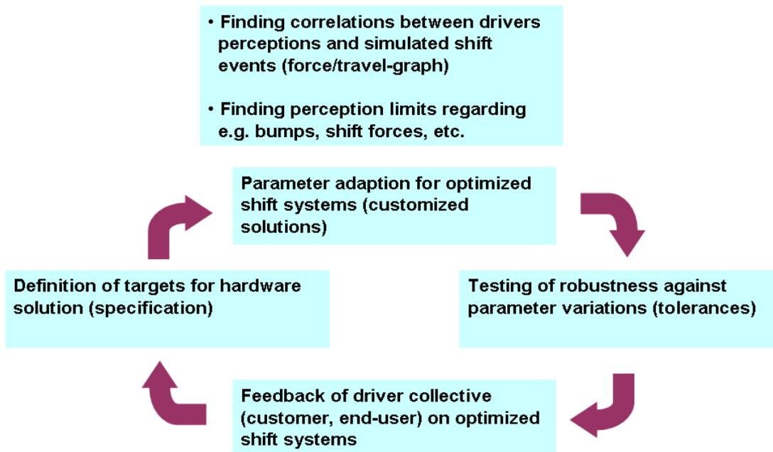
Figure 5: Development process using the shift simulator
