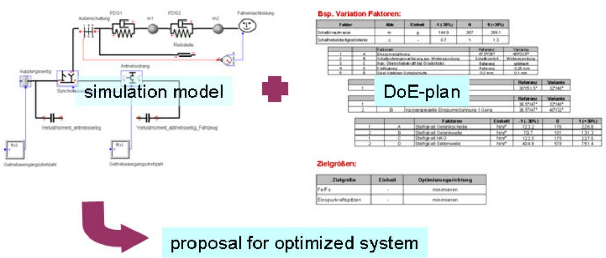
Figure 4: Application of simulation for shift system optimization
