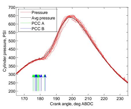
Stable main chamber combustion due to perfect PCC firing
