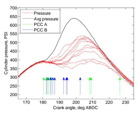
Slow and late main chamber combustion due to delayed PCC firing
