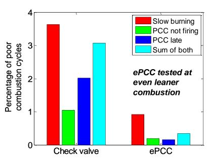
⇒The real solution is a pre combustion chamber with electronic fuel injection
