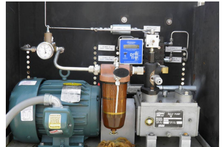
New lubrication system with divider block
