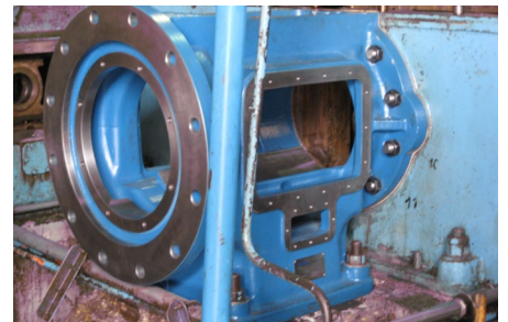
Crosshead guide installed on the compressor
