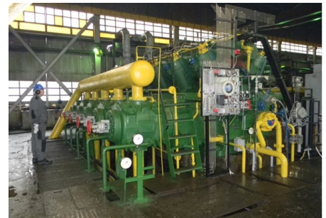
Integral compressor in new condition, with 5 compression and 10 power cylinders
