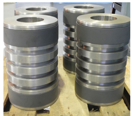
Modified pistons with shrink-fit rider rings
