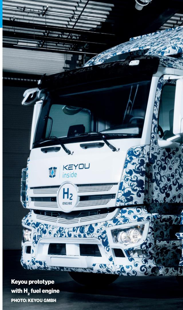
**Keyou prototype with H<sub>2</sub> fuel engine**
