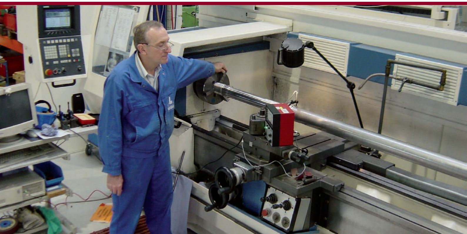
Piston rod reconditioning
